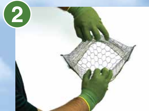
2 Flatten out bottom fold
