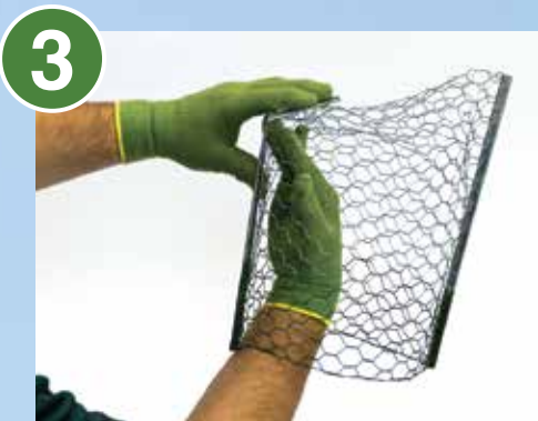
3 Bend side seams flat against bottom
